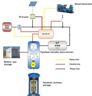
Figure 5 - SmartBox MicroGrid typical configuration
